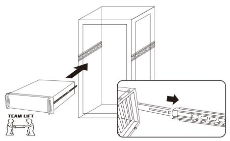
Slide the server chassis into position by aligning and sliding (R1) onto the slide rail (R2) and (R3) on the rack.
