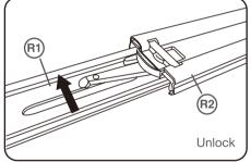
Pull (R1) all the way out to its maximum slide position. Locate and release the locking lever by sliding it upward. This will release (R1) from (R2).
