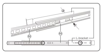
Install the outer rail (R3) on to the L-bracket using M4 Screw pack . Now the L-bracket, (R2) and (R3) should be well installed on the rack.
