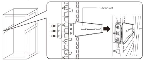
Install the L-bracket on the cabinet frame using M5 Screw Pack &M5 Washer.
