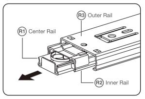
The slide rail is consist of three rails: (R1) Center Rail, (R2) Inner Rail, (R3) Outer Rail
